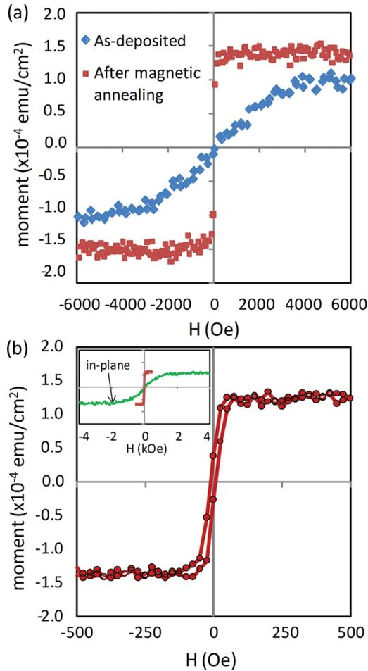
FIG. 1. (Color online) (a) Out-of-plane magnetization curves for a 15 Å CoFeB film before and after magnetic annealing (b) Out-of-plane magnetization curve for the annealed CoFeB film in a smaller field range. The corresponding in-plane magnetization curve is inset.
