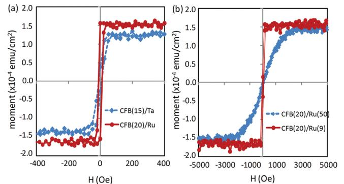
FIG. 3. (Color online) (a) Out-of-plane magnetization curves of CoFeB(15)/Ta and CoFeB(20)/Ru(9)/Ta films (thickness in Angstroms). (b) Out-of-plane magnetization curve of CoFeB(23)/Ru(9)/Ta. The corresponding in-plane magnetization curve is inset.
