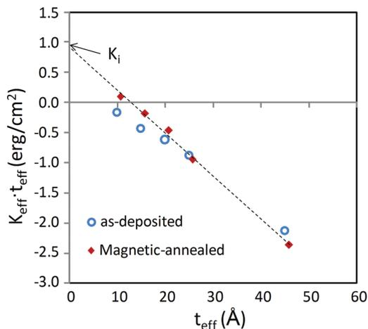
FIG. 2. (Color online) Magnetic anisotropy energy ( $K_{\text{eff}}$ ) times the CoFeB thickness ( $t_{\text{eff}}$ ) vs  $t_{\text{CFB}}$  for as-deposited and annealed CoFeB films.
