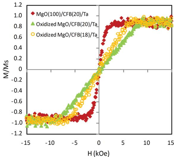
FIG. 4. (Color online) Out-of-plane magnetization curves of single-crystal MgO(100) substrate/CoFeB(20)/Ta and Si substrate/Ta buffer/oxidized MgO/CoFeB(18 or 20)/Ta
