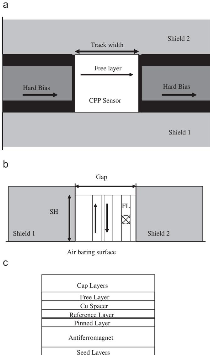
Fig. 2. Schematic representations of a CPP GMR read head sensor. (a) an air baring surface view of the sensor where the insulating layer between the hard bias and the sensor is drawn in black. (b) device cross-section highlighting the relative orientations of the free layer and antiparallel-pinned layers. (c) Generic CPP GMR sensor stack. The dark line separating the pinned and reference layers is the thin Ru coupling layer.
