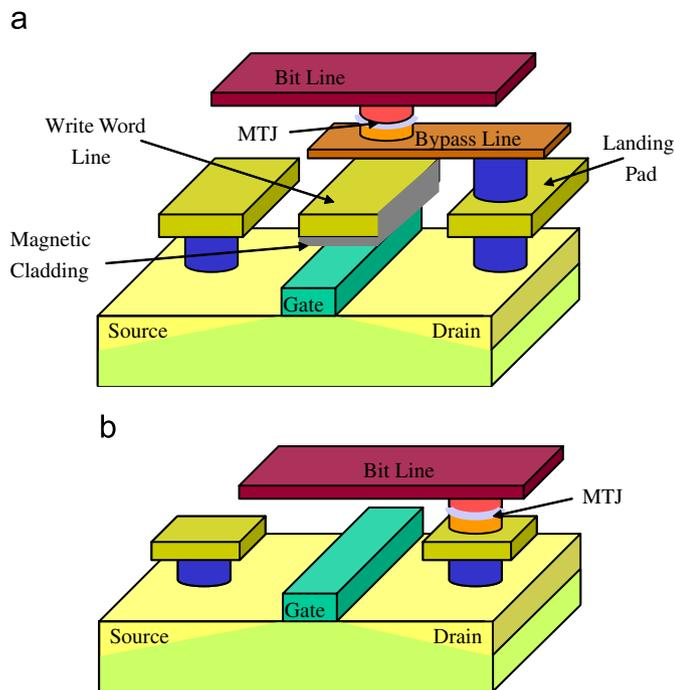
Fig. 4. Comparison of conventional toggle field-switched MRAM cell (a) and ST-MRAM cell (b). The ST-MRAM eliminates the need for a remote write line and a bypass line, allowing for a more compact architecture [56].
