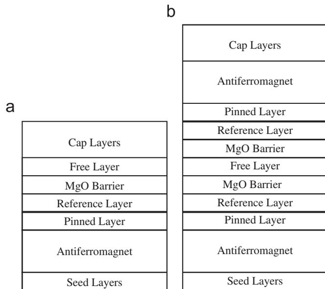
Fig. 5. Schematic representation of a simple (a) and dual (b) MRAM stack. Unlike Fig. 3, the pinned layer magnetizations in the dual stack are oriented anti-parallel to one another.
