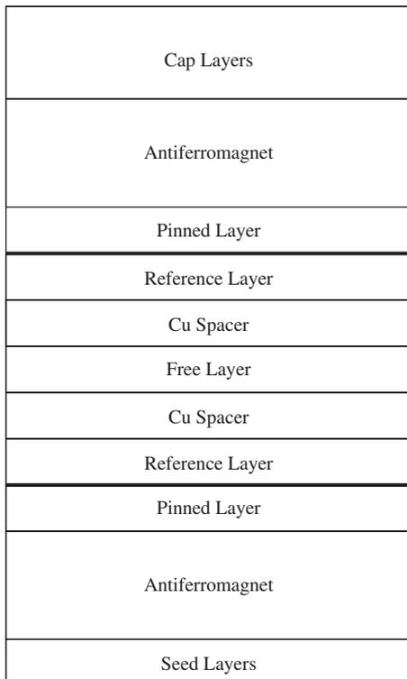
Fig. 3. Schematic representation of a generic CPP GMR dual sensor. The pinned layer magnetizations are set parallel to one another.
