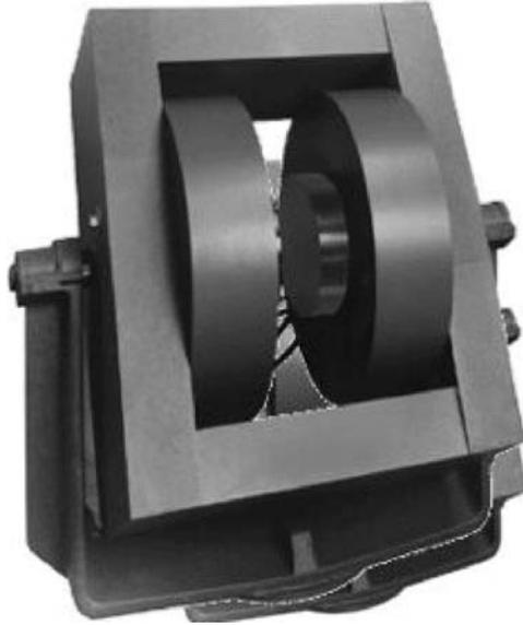
Electromagnets consist of field coils to polarize an iron core, a yoke to guide the flux and pole pieces to concentrate flux in the airgap, Fig. 12.11. Flux guidance and concentration in electromagnets requires material with the highest polarization and very little remanence. Pure soft iron or  $\text{Fe}_{65}\text{Co}_{35}$  is used. For best results, the pole pieces are tapered at an angle of  $55^\circ$ .
